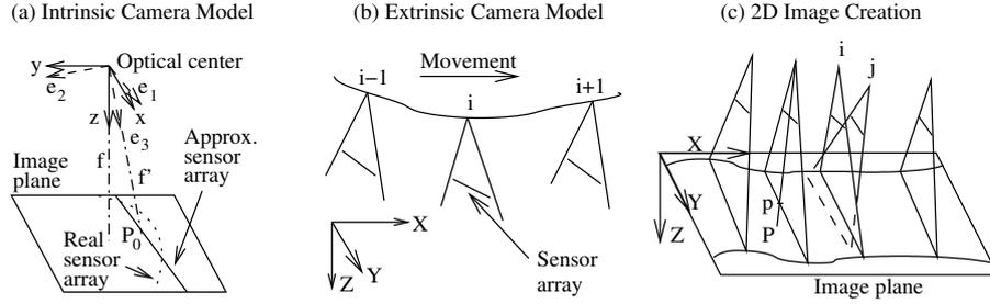
**Fig. 2.** Camera model and the creation of a corrected 2D image.
