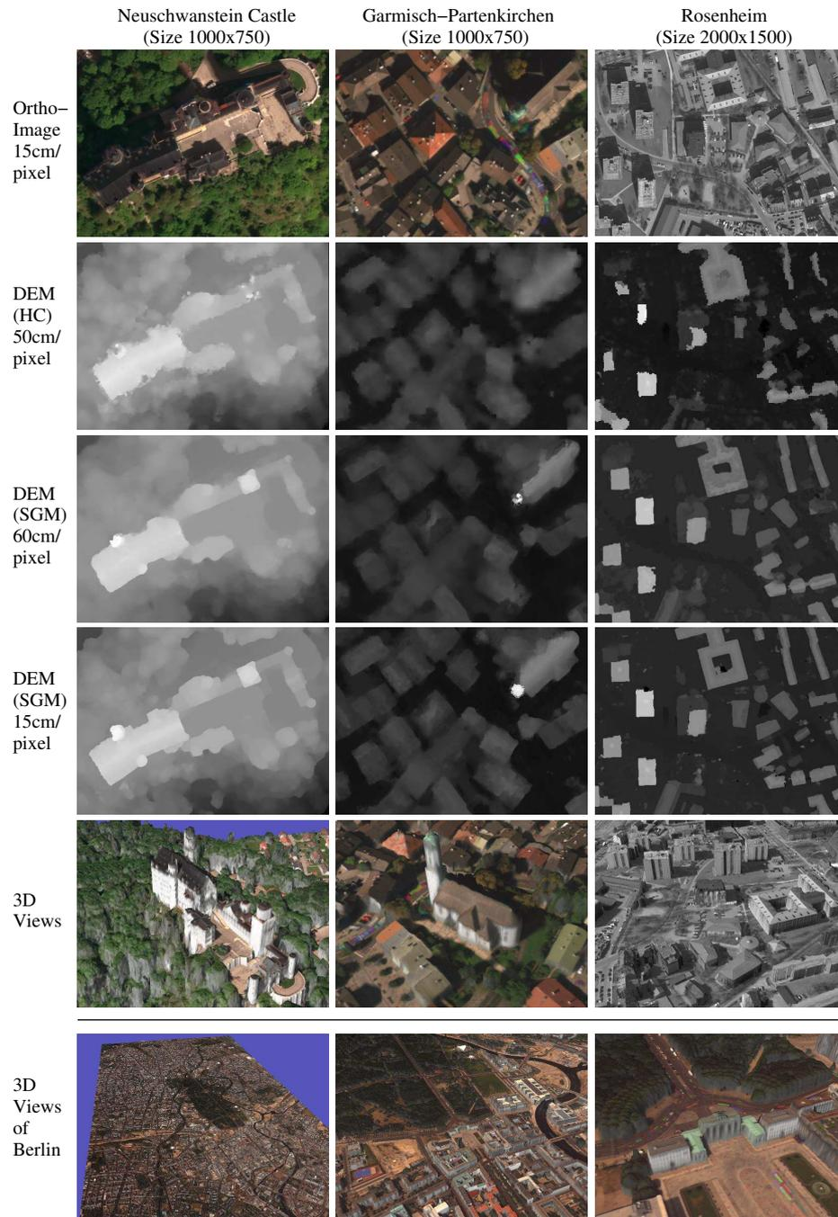
**Fig. 4.** Results of a hierarchical, correlation base method (HC) that finds correspondences within a 2D area and the SGM method that finds correspondences along calculated epipolar lines.
