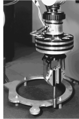
Figure 3c: Endeffector in starting po- sition at the contour to be followed
