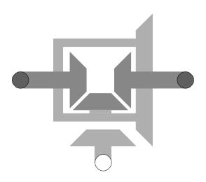
A differential gear can be regarded as a special case of the planetary gear. The planetary gear essentially consists in three gear wheels, the ring wheel, the sun wheel and the planet wheel. The planet wheel occurs mostly multiple times, but that is irrelevant for the kinematics. Relevant is the ratio of teeth of the ring over the sun teeth.
