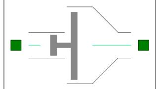
Hydraulic transformer with gain M[1]
