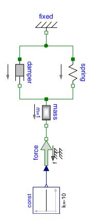
This pretty much prescribes the analog electric circuit. The only difference is the different design of mass and capacitor. The mass in implicitly "grounded" The capacitance is not. The mass is designed as two port element but just for the sake of convenience. The two ports express the same pair of variables, there is no difference of the potential variable across the mass element.
