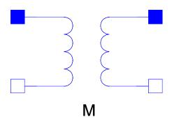
Electrical transformer with gain M [1]
