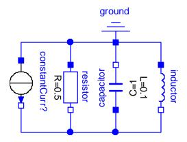
All components of this circuit share the same difference in voltage potential. There is also the dual circuit, where all components share the same current that expresses the velocity of the mass.
