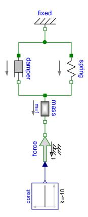
It represents a mass attached to a spring-damper pulled by a force. The following parameters are applied: mass = 1 kg, spring coefficient = 10 N/m, damping coefficient = 2 N/m, force = -10 N, initial position of the mass = 0 m.
