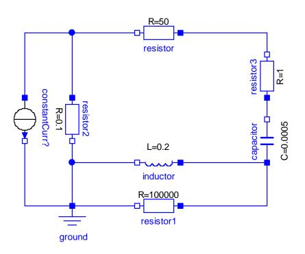
On top, you see a simple RLC-Circuit where with a few extra resistors that make the ideal components more realistic. Your task is to derive the state-space form of this circuit.
