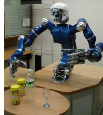
Fig. 1. The DLR humanoid two-arm system "Justin", the target system for the task planning approach.
