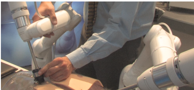
Fig. 1. Soft robotics enables hands-on the MIRO for insertion of the minimally invasive instrument into the patient.
