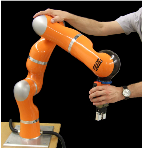
Figure 1: The new KUKA Lightweight Robot (right) is designed for direct physical interaction with humans. Contact scenarios in physical Human-Robot Interaction (right).
