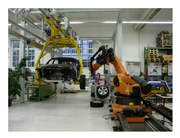
Fig. 1. Set-up at iwb for mounting wheels to a moving car body.
