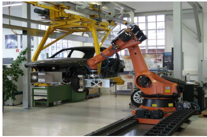
Fig. 1 (a) Setup for wheel assembly
