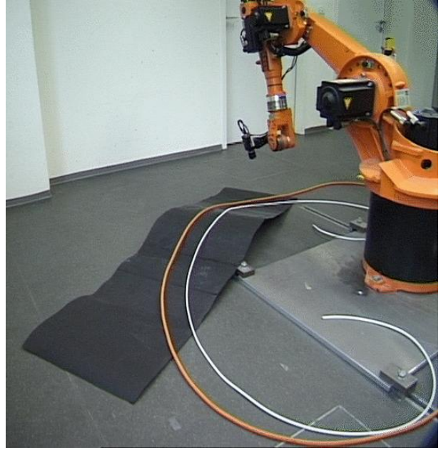
Figure 9: Experimental setup with KUKA KR6/1 industrial robot and endeffector mounted camera
