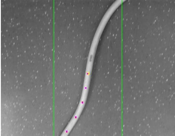
Figure 7: Displayed camera image with markers representing the used window, the image center, and five detected line points
