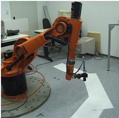
Fig. 2. Robot and edges for visual servoing
