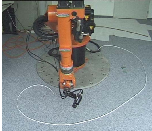
Figure 4. Originally the robot is programmed to execute a quarter of a circle around its base, back and forth. Image data of the robot-mounted camera are used to modify the radial distance in order to track the wire.
