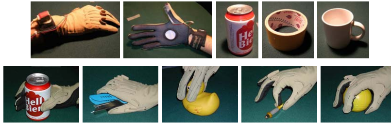
Figure 6: (above) The devices and some of the objects used for the experiment, left to right: the CyberGlove, the Force Resistor Sensor attached to the subject's thumb, the beer can, the duct tape roll and the mug. (below) The 5 grasp types to be recognized, left to right: power large, power flat, tripodal precision, thumb/index precision and spherical precision.
